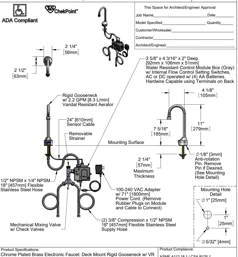
Chrome Plated Brass Electronic Faucet: Deck Mount Rigid Gooseneck w/ VR Aerator, AC/DC Control Module w/ Internal Flow Control Setting Switches, Temperature Control Mixing Valve w/ Check Valves, 18" Hot & Cold Supply Stop Flexible Connector Hoses
